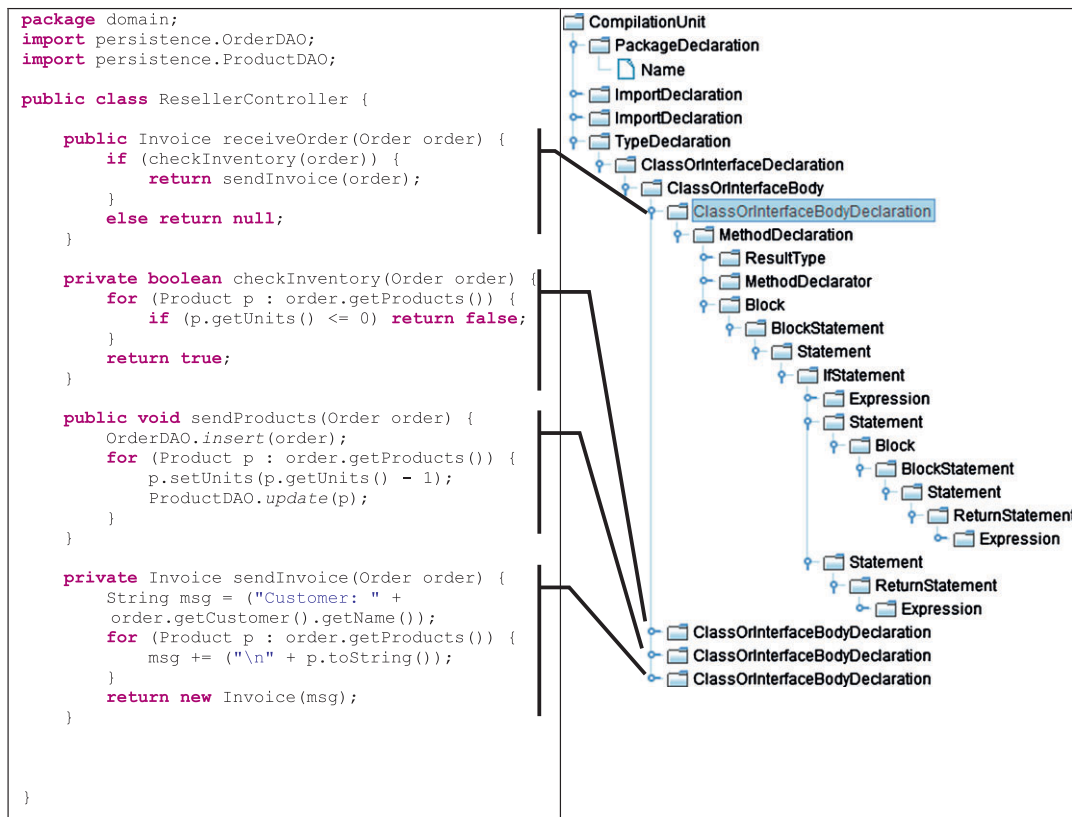
Figure 4. An example of the L0-to-L1 transformation for a product shipping system.
